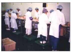
molded grating and grating rubber feet, any size work mat can be created. The feet raise the grating 13mm above the ground and the open mesh allows chips and fluids to fall below the standing surface providing a safe, clean working area. Should your operations require more complex work stations, Fibergrate's turnkey approach includes design, fabrication and installation services for everything from a simple portable station to larger fixed platforms with railings and stairways.
